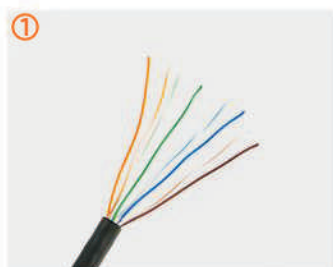
① Separate the wires
